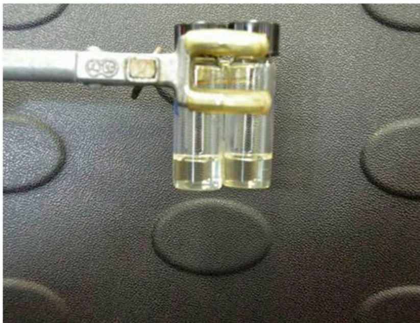
Figure 2. ENB(97.5%)/DCPD(2.5%) and ENB(95%)/DCPD(5%) after 1 h at -50\text{ }^{\circ}\text{C} .
